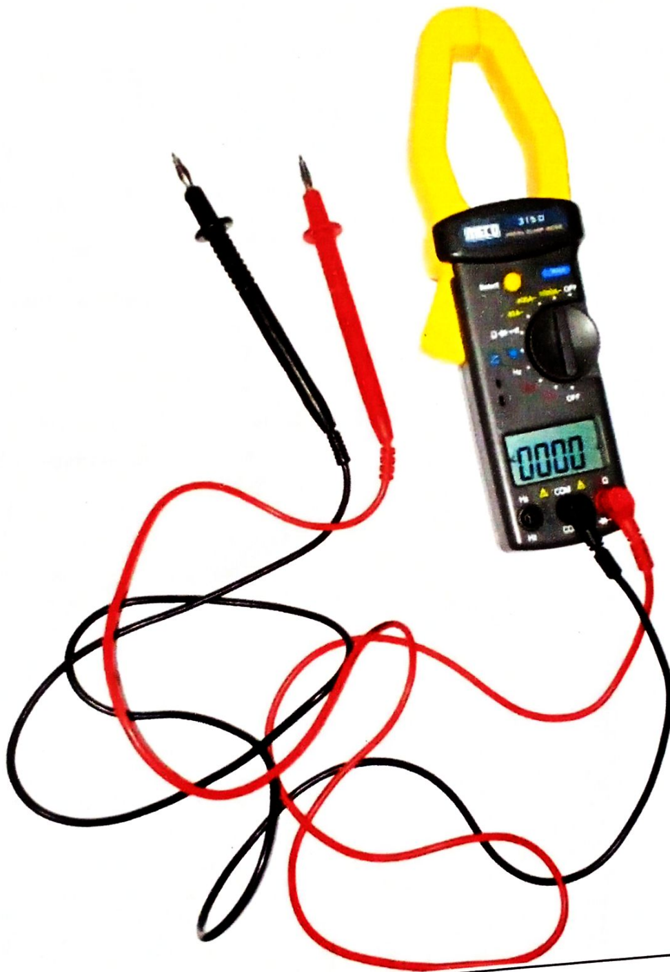
Picture 1 MECO 3150 DIGITAL CLAMP METER
