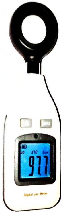
Picture 3 Nishant NE 1010 Lux meter
